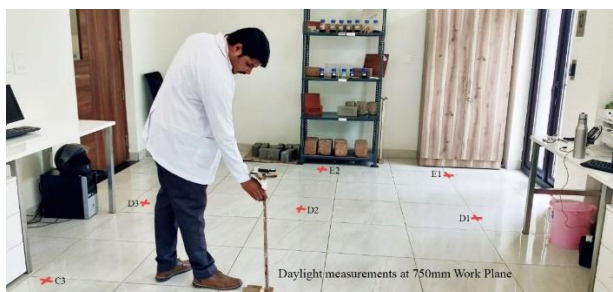
Figure 10 Measurements of illuminance levels using a Illuminance Meter at the MTCoE lab test bed.
